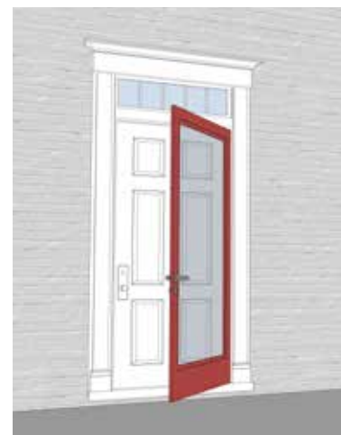
This storm door is a single panel which allows the historic door to be seen.
