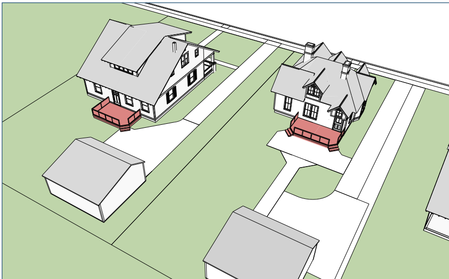
Examples of decks added to the rear of historic houses. The view on the left shows the rear location while the view on the right shows the minimal visual impact of the added deck on the historic front view of the house.
