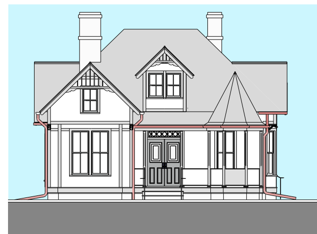
A properly installed gutter system will ensure the removal of water through the downspouts and away from the buildings.
