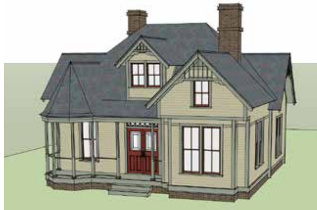
A Queen Anne style house typically has a wall color, trim color, and accent color for window sash and doors. An additional color may be used to further accent the building.
