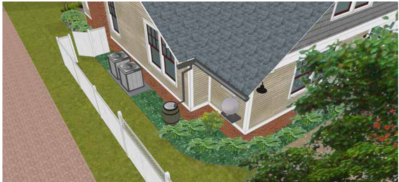
HVAC equipment should be screened with landscaping and fences.
