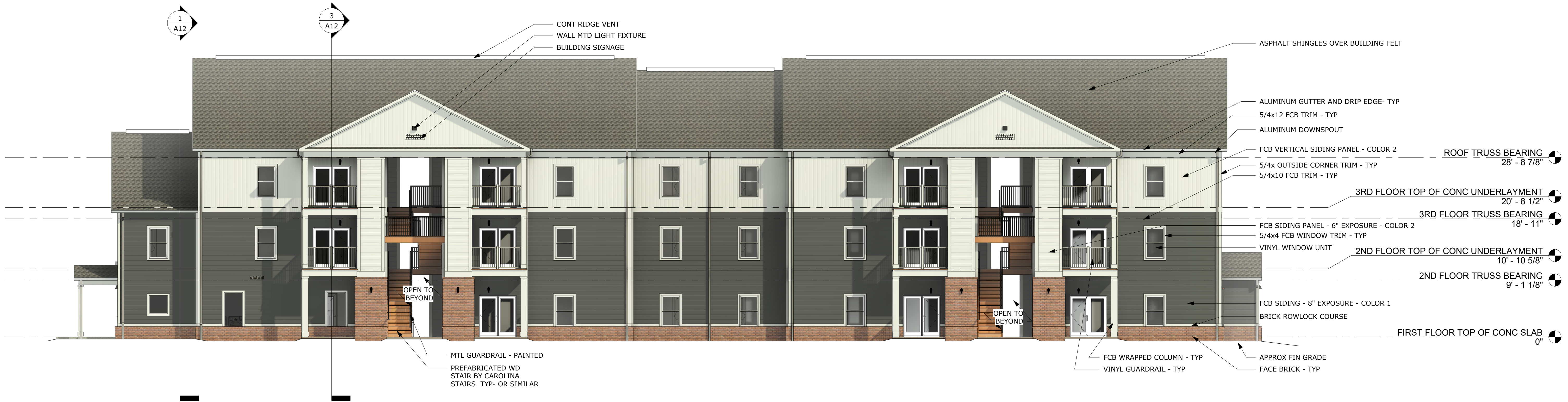
1 BUILDING B - NORTH ELEVATION RENDERED A10 1/8" = 1'-0"
