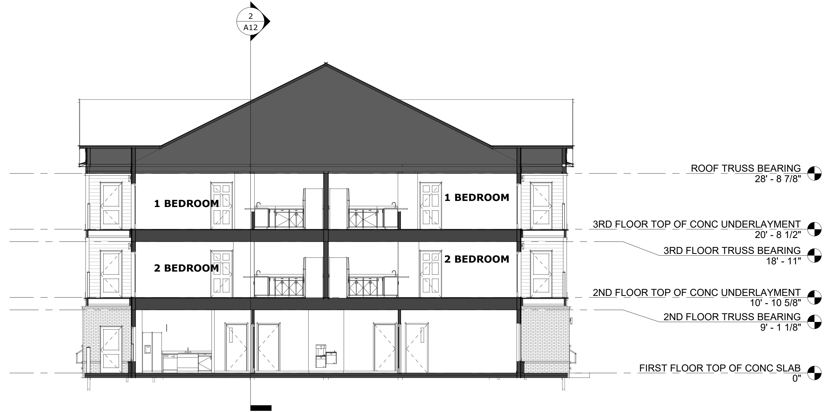
3 BUILDING 'B' 3-STORY BUILDING SECTION Copy 1 1/8" = 1'-0"
