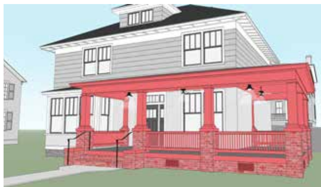
Foursquare houses in Davidson feature asymmetrical full porches.
