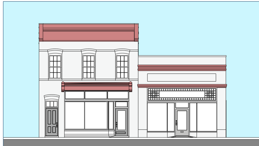
Most commercial buildings have a cornice at the storefront and roof line. Materials can range from brick to metal to wood.
