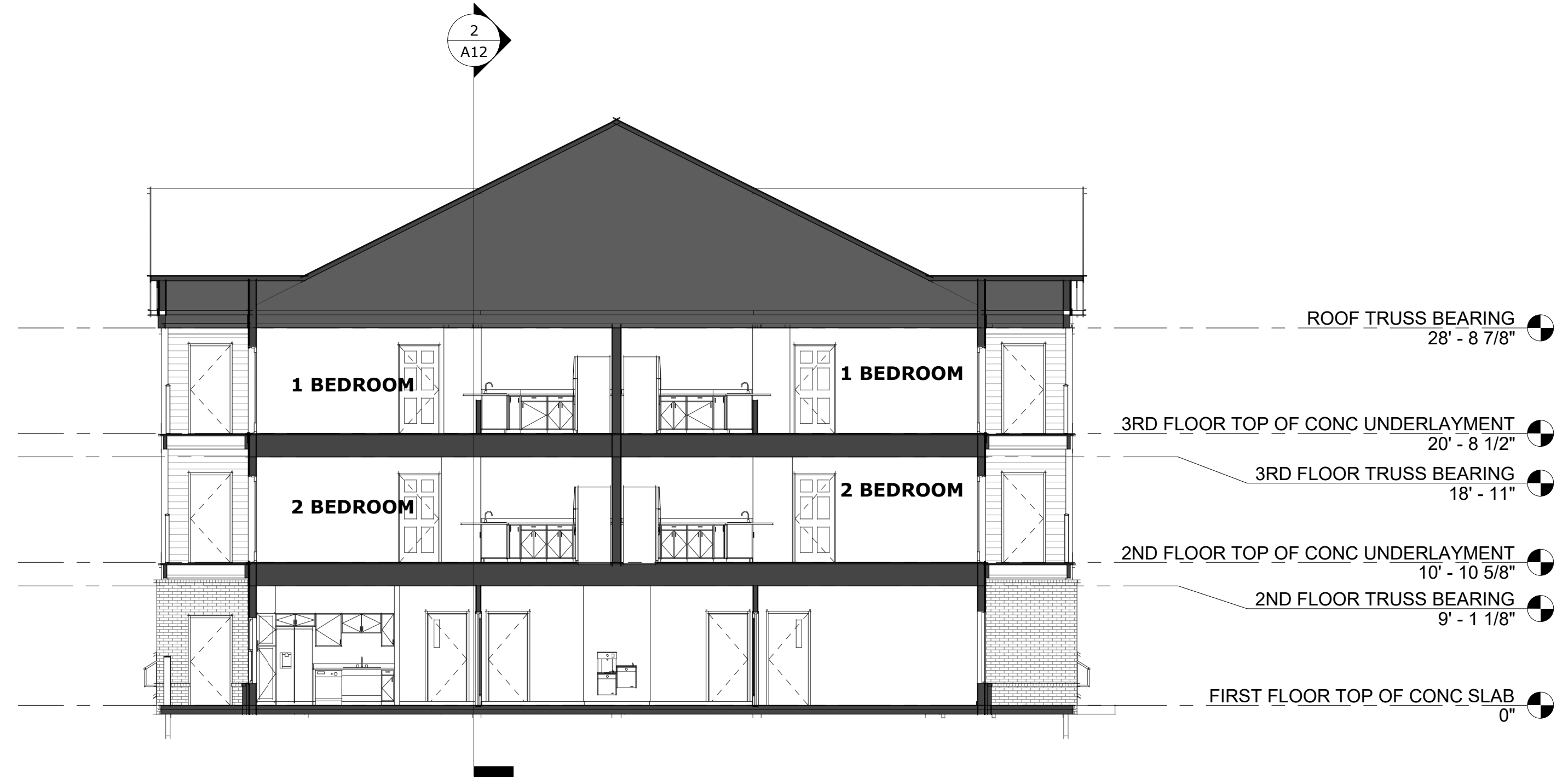
3 BUILDING 'B' 3-STORY BUILDING SECTION Copy 1 1/8" = 1'-0"
