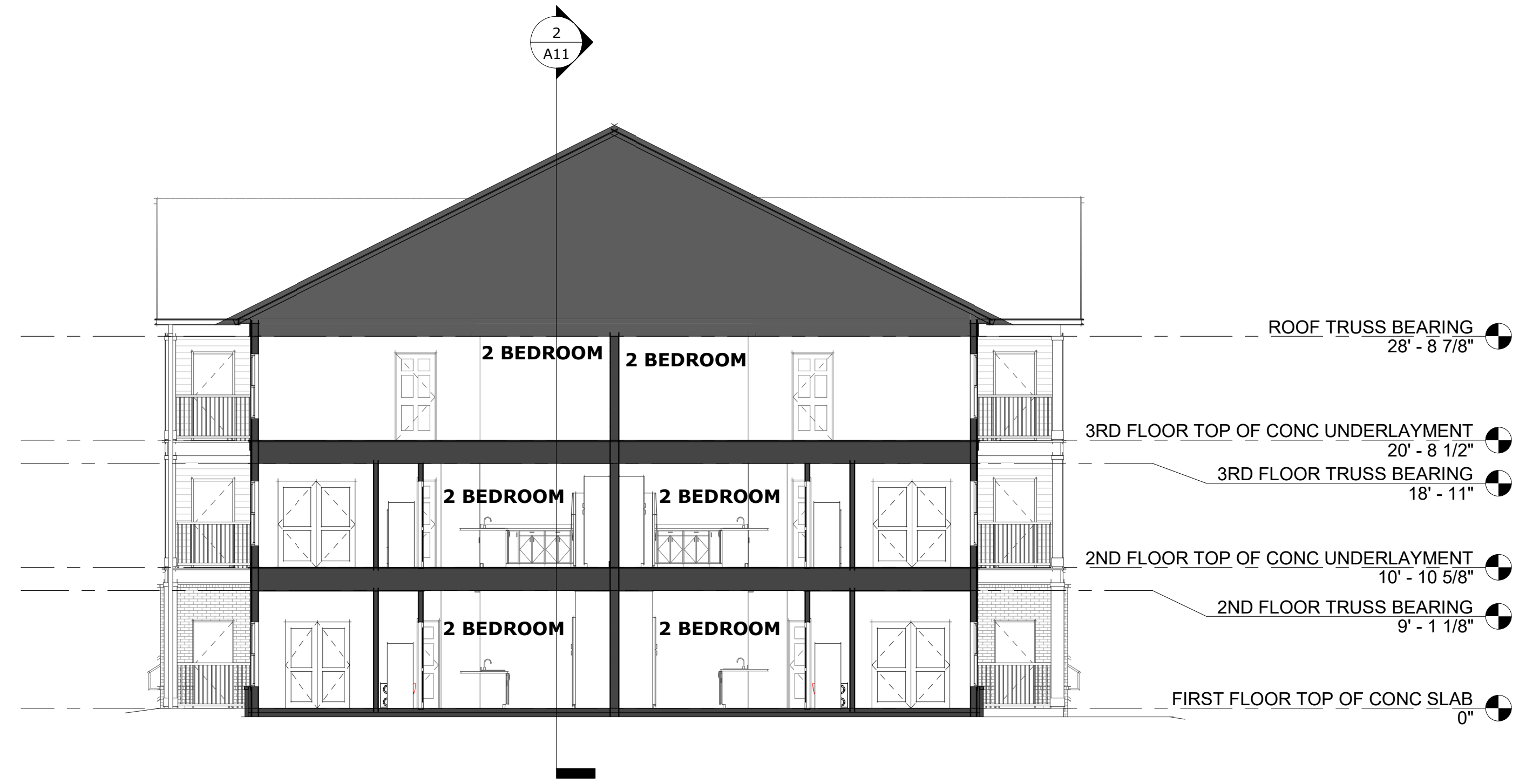
3 BUILDING 'A' - TRANSVERSE SECTION A11 1/8" = 1'-0"
