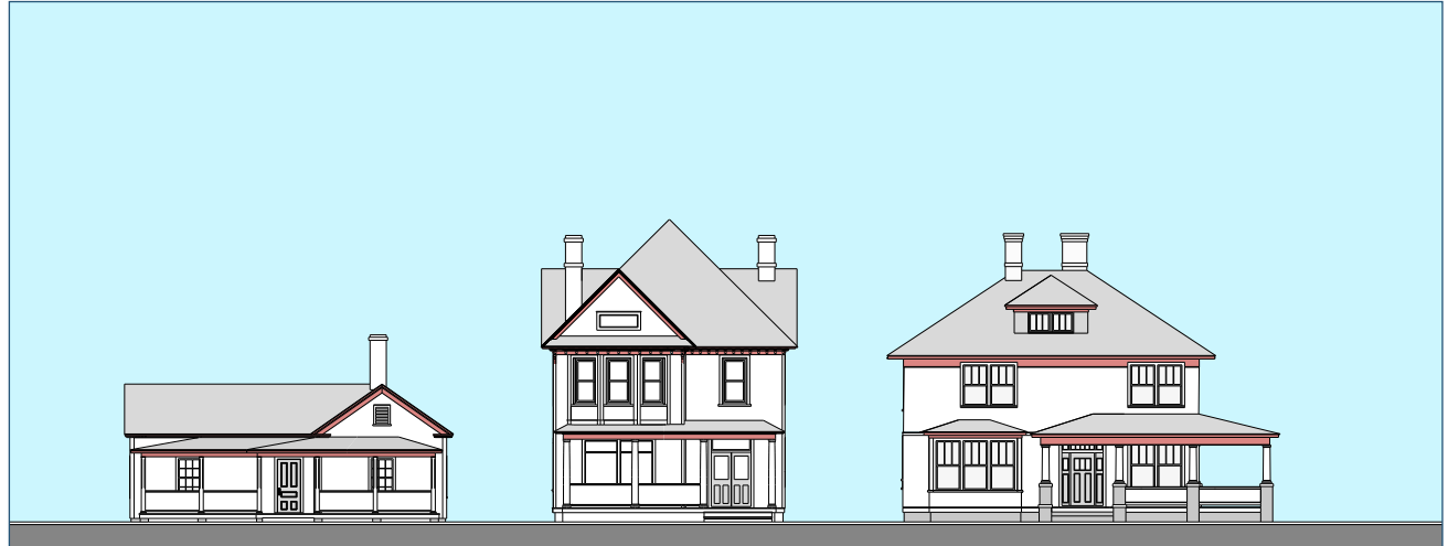
Residential buildings typically have cornices at the roof line and porches. The material is generally wood and the design is based on the complexity of the style of the building.
