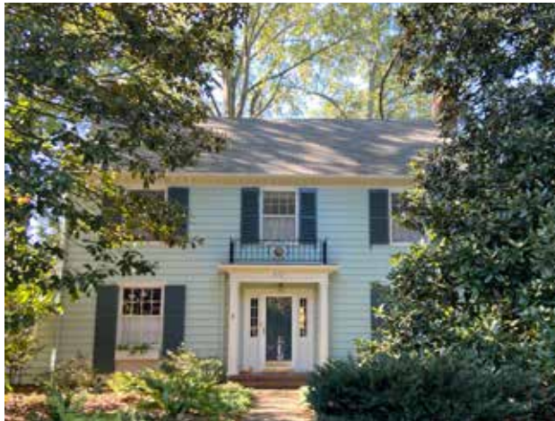
This Colonial Revival home has a typical central entry portico supported by Roman Doric columns
